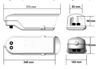
MAXIMUM INTERNAL DIMENSIONS 250mm Length x 110mm Width x 70mm Height
